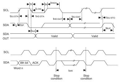
Note: The write cycle time  $t_{WR}$  is the time from a valid stop condition of a write sequence to the end of the valid start condition of sequential command.
