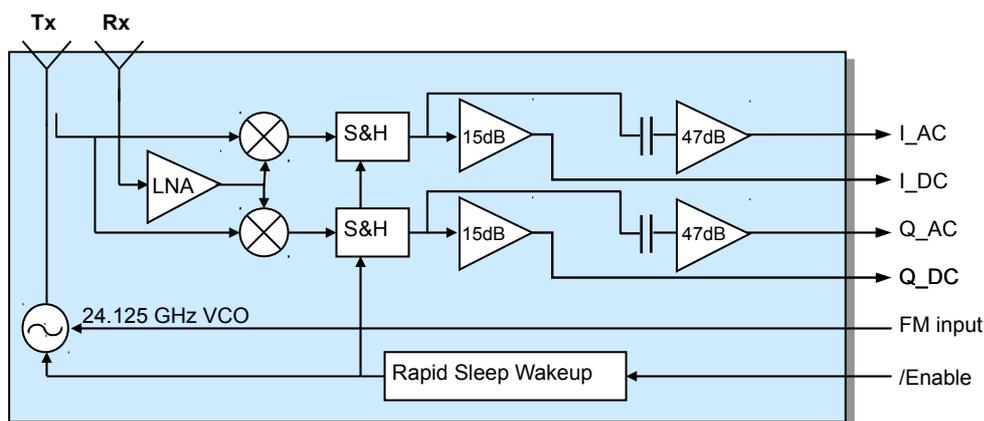
Fig. 1: K-MC3 Blockdiagram
