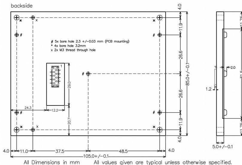
Fig. 4: Mechanical dimensions
