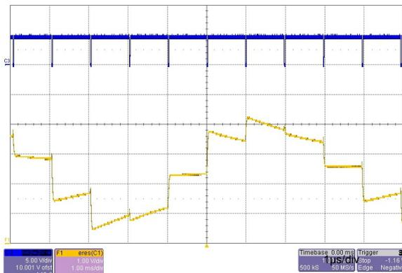
Sampling signal ( $t_c = 1\text{ms}$ ,  $t_{\text{on}} = 7\mu\text{s}$ )
