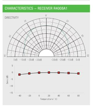
**NICERA offers a new series T/R4008A1** of ultra small ultrasonic sensors at frequency 40 kHz. The diameter is 8 mm only at similar sound pressure level as sensors with larger diameter. This allows miniaturization of ultrasonic applications.
