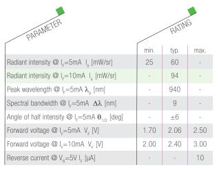
The **IRP3016L24-B2** is a GaAs infrared LED in a small SMD package with tight viewing angle of  $\pm 6^{\circ}$ . The device has a peak wavelength of 940nm LED spectrally matched with phototransistor or photodiode.
