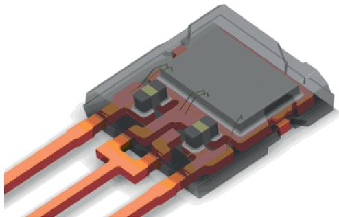
The direct-angle Hall-effect sensors HAC37xy from Micronas are suitable for multi-dimensional magnetic field measurements in automotive and industrial applications. The TO92UF package was especially designed for this new sensor and integrates both a chip from the HAL37xy sensor family based on Micronas' 3D technology as well as two capacitors up to 100 nF.
