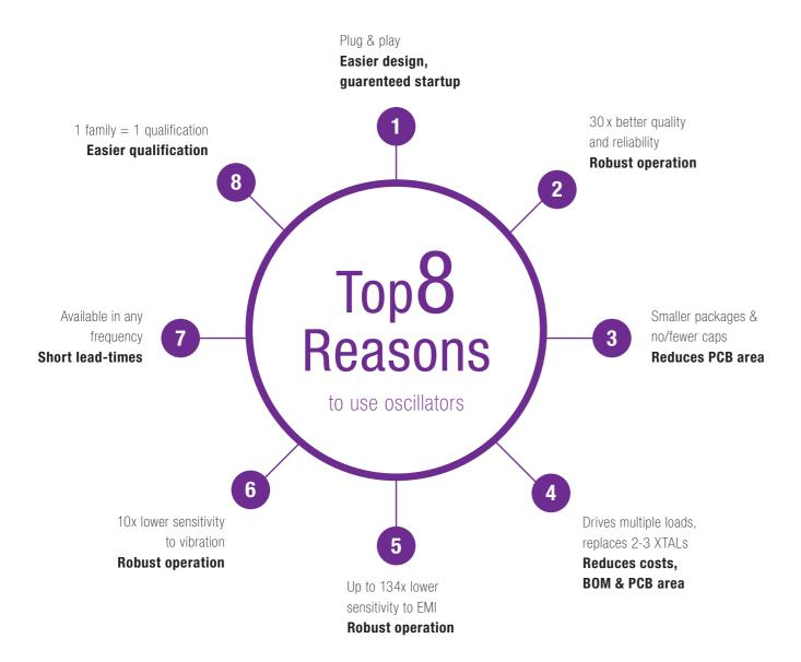
SiTime has many components that are pin-compatible with the quartz-based Oscillators with the advantage of being immune to shock & vibration and consuming little power. Bosch manufactures the MEMS resonators in Reutlingen, the wellknown companies in Asia handle the analog ICs and packaging in different places. Using multiple fabs ensure that even in a critical situation the supply chain remain stable.
