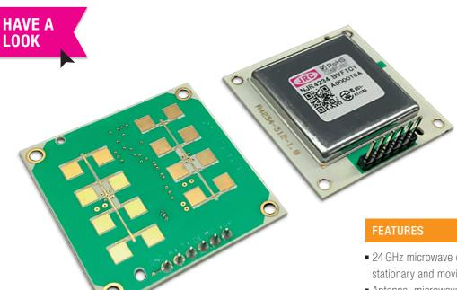
The NJR4234BW is a sensor module that can measure the distance to stationary as well as to moving objects such as a pedestrian up to 30 m ahead.
