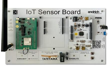
Cortex® M23 or RISC-V microcontrollers converting them to an IoT end point with sensing and communication capabilities. Endrich is providing this conceptual development infrastructure as a platform, not as a product, we still live on component sales, but supplement it with development support sharing reference circuit design, software code and providing access to our cloud database during the product development.
