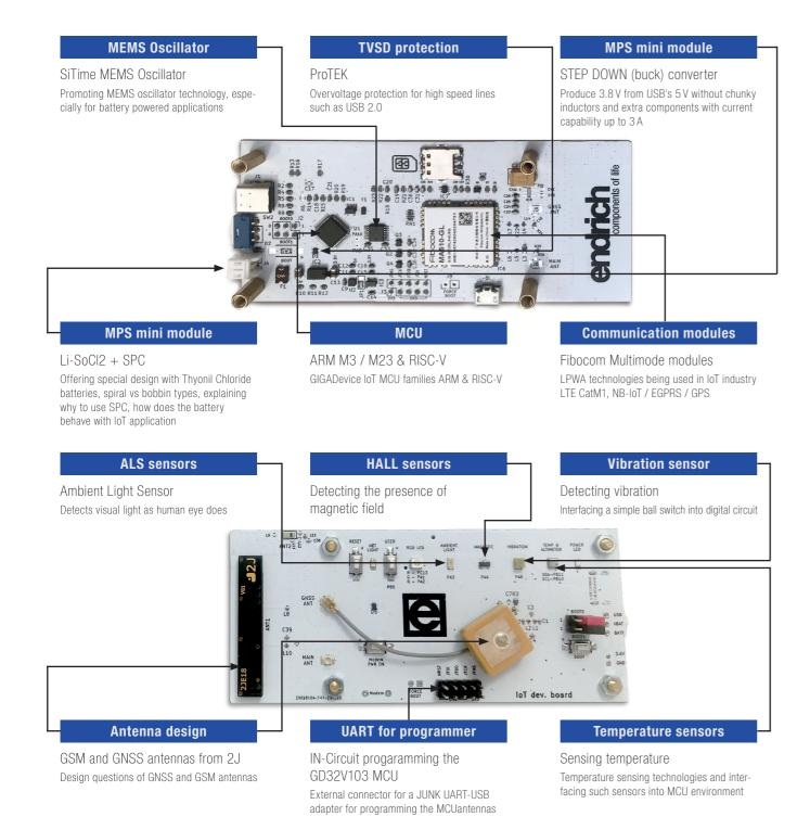
The IoT board acts as a development evaluation board for the IoT technology. Can be used as MCU evaluation, GSM modem evaluation. For this purpose, external connectors are available for the MCU and the Modem UART interfaces
